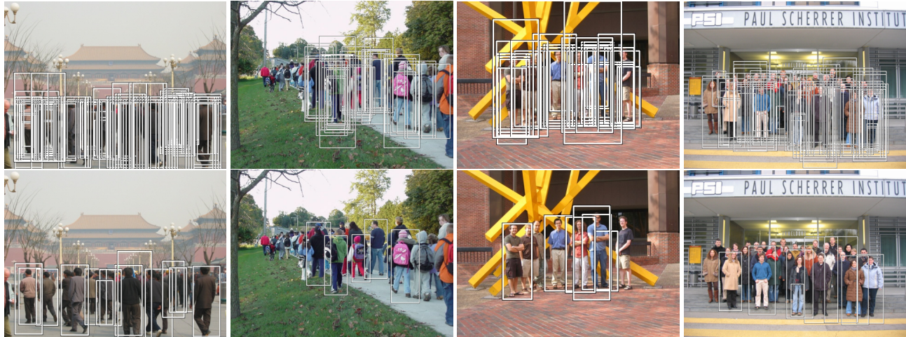
Figure 6: Detection examples on random internet images. Top : raw detection results. Bottom : merged detection results using mean shift clustering technique.
